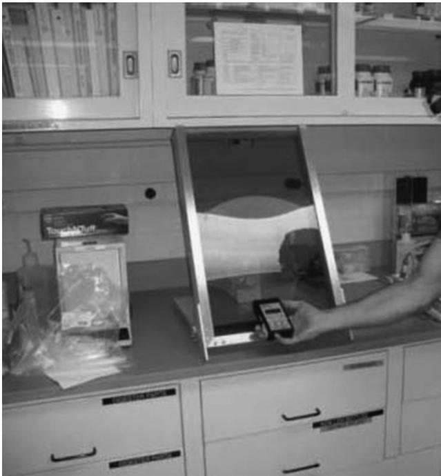
**FIG. 8.** Table top shield used at LaSalle Nuclear Power Plant (reproduced with permission from Exelon).
